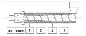
Type:45/25d(L/D=25) Screw compression ratio =3:1,
