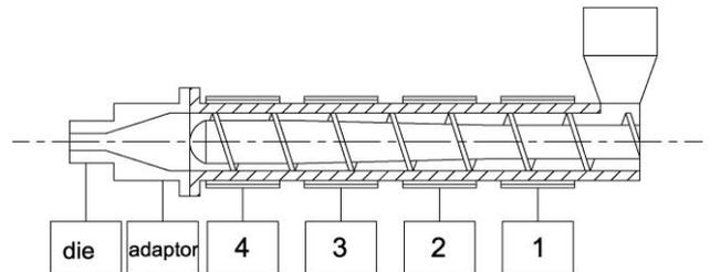
Type:45/25d(L/D=25) Screw compression ratio =3:1,
