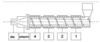
Type:45/25d(L/D=25) Screw compression ratio =3:1,
