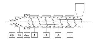
Type: screw: 45mm, L/D:b30, compression ratio 3:1
