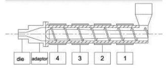
Type:45/25d(L/D=25) Screw compression ratio =3:1,
