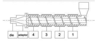
Type:45/25d(L/D=25) Screw compression ratio =3:1,
