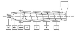
Type: screw: 45mm, L/D: 30, compression ratio 3:1
